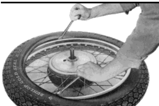
FIG. F12. Removing the first bead.
